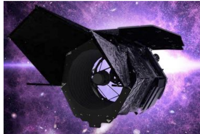
Nancy Grace Roman Space Telescope Hubble resolution with ~100x larger field of view
